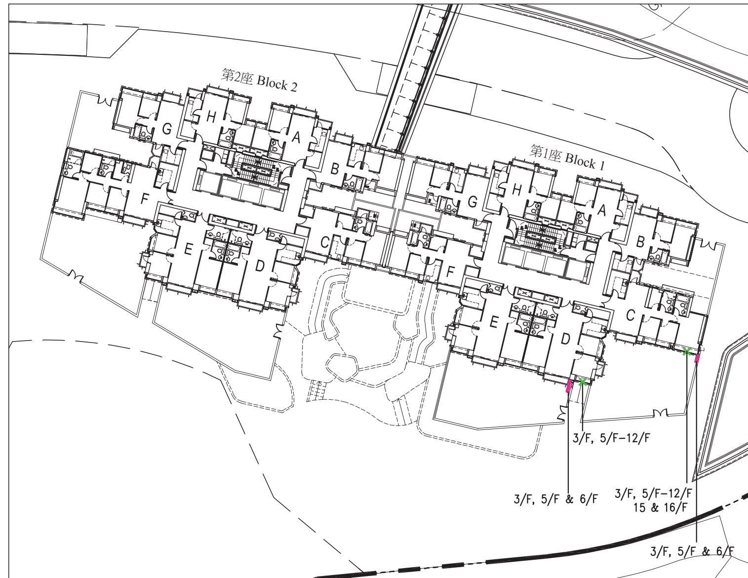
垂直建築鱗片及固定玻璃窗相對於個別住宅物業的位置 Locations of Vertical Architectural Fins and Fixed Window at respective Residential Units
